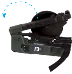
Step 1 Release arm strap and pivot shaft
